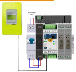
Raccordement TIC, bornes I1 I2
